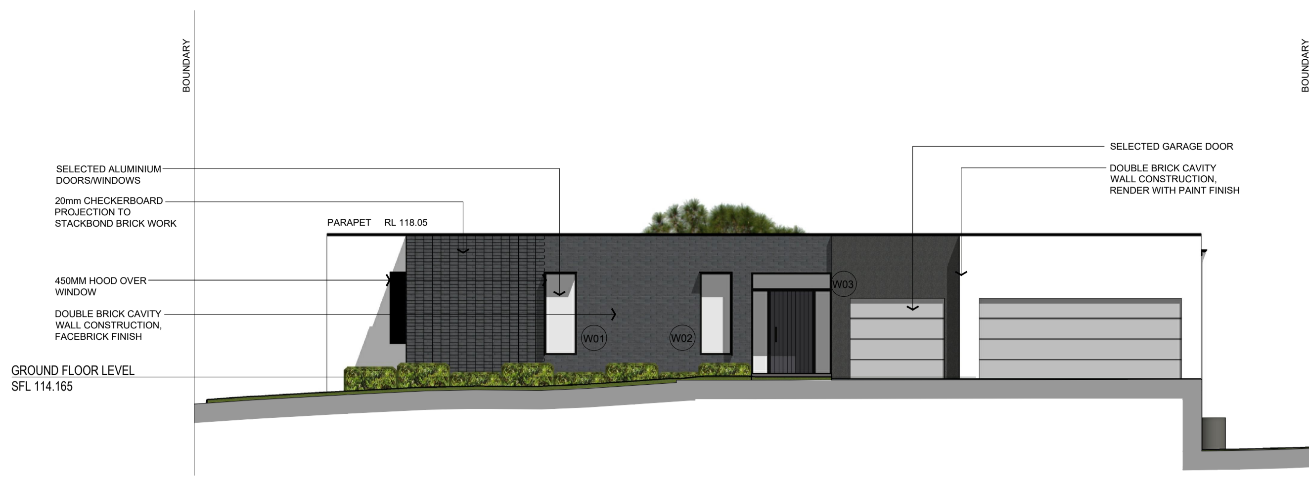
1 STREET ELEVATION (NORTH) SCALE 1 : 100 @ A1
